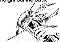
Attach exhaust duct to each dryer duct. Then connect exhaust ducts to exhaust hoods or main exhaust. Use duct tape to seal all Joints.
